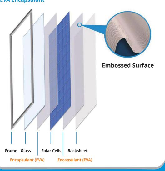
'CONSERV A UVT - 14 FC' is a wide process window curable, UV stable and weather stable Ethyl Vinyl Acetate (EVA) PV Encapsulant proven for single stage as well as short cycle multi stage lamination processes. It is an UV transparent PV Encapsulant used as top layer towards the glass for all Crystalline PV Modules. It allows PV Modules comprising blue - light sensitive PV Cells of a given efficiency, to generate higher power.
