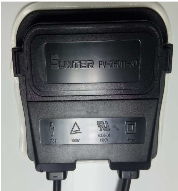
Junction Box Close View
