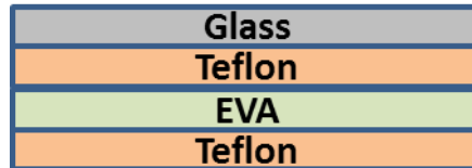
Fig (1): Laminate structure for Cured EVA sheet sample preparation
